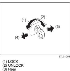
• Turn the lock knob forward, then pull and hold the door handle as you close the door.
